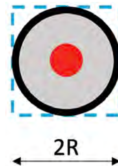
Figure 48 Shield in box shaped arrangement
